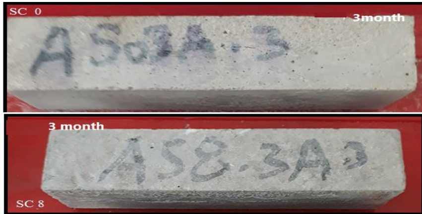
Figure 9. Geopolymer Mortar After 90 days of Exposure to MgSO 4 for SC and WC.
