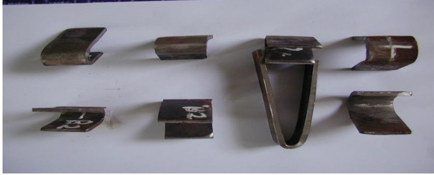
Figure (4) Bend Test for the samples (X1 to X3,) Cylinders
