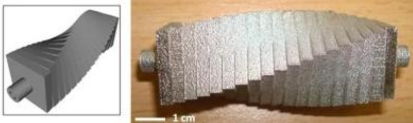
Figure 1: Showing poor surface finish
