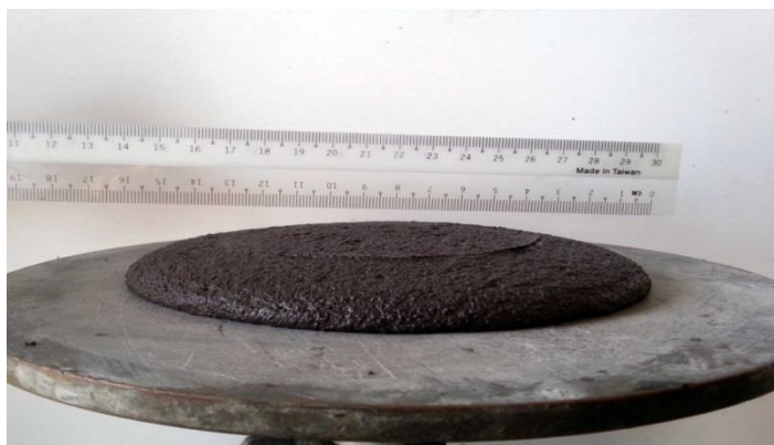
Figure 4: Flow table used to measure the workability of TPOFA-based geopolymer mortar
