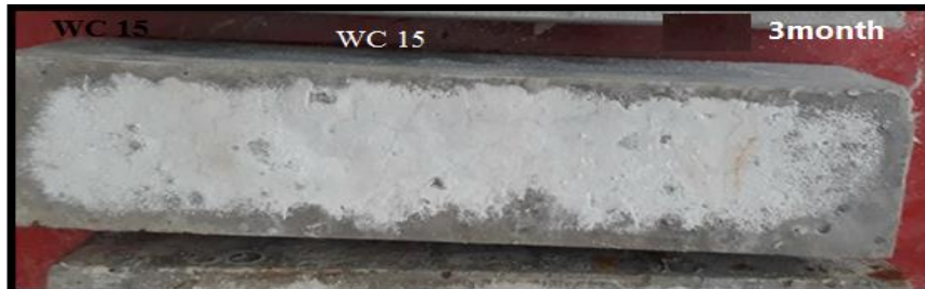
Figure 10. Geopolymer Mortar After 90 days of Exposure to MgSO 4 for WC.
