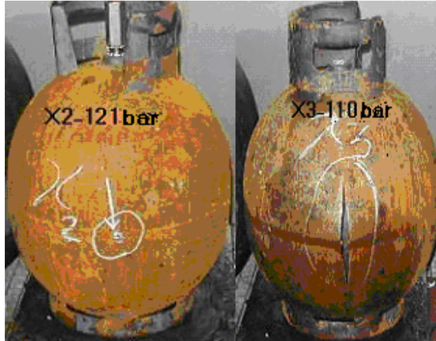
Figure (5) Burst shape of the (X) samples which have been selected and subjected to the burst pressure
