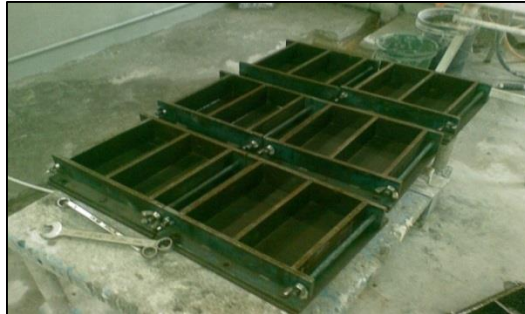
Figure 5: Bricks mould of 215mm x 100mm x 65mm
