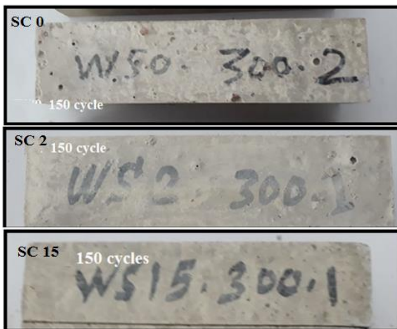
Figure 2. Geopolymer Mortar after 150 cycles for SC.
