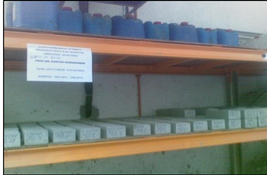
Figure 7: Air dried of samples at the ventilation area
